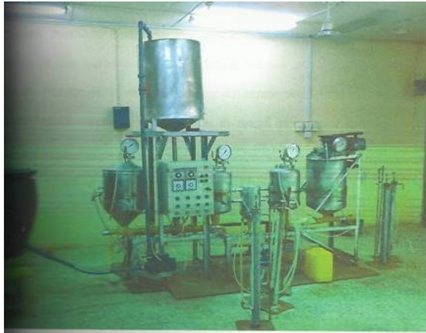
Figure 3.8 Fabricated pilot scale of the integrated assembly of three different bioreactors, UASB, UBCSD and CSTR (Agulanna 2012).
