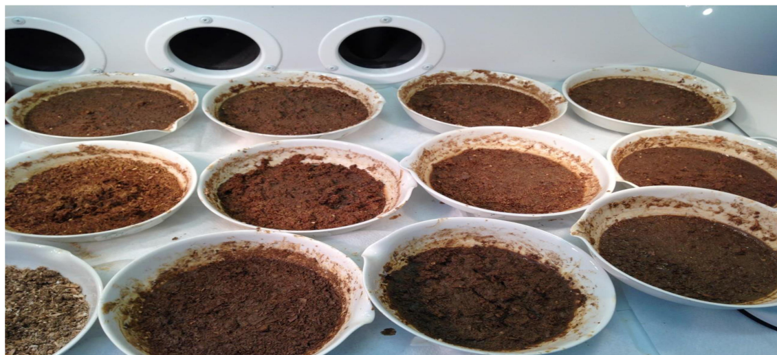
Fig 3.1: The mixture of contaminated soil +( poultry+cow+sawdust) manure
