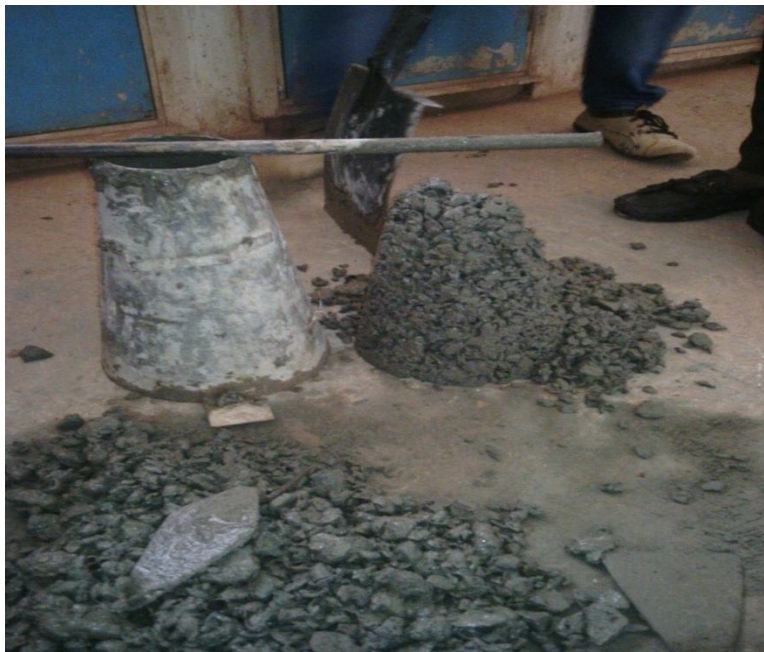
Plate 3: Slump test to determine workability of palm kernel shell concrete
