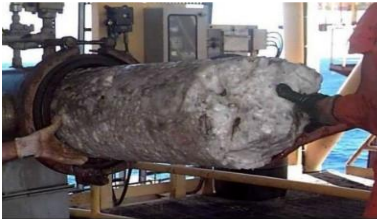
Fig 2.1: A large gas hydrate plug formed in a subsea hydrocarbon pipeline.
